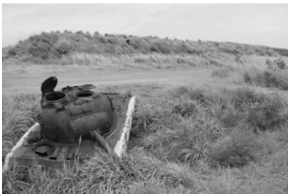
Figure 6: A disabled Sherman tank. Note the concrete attached on both sides of the tracks to counter attachment of magnetic bombs.
